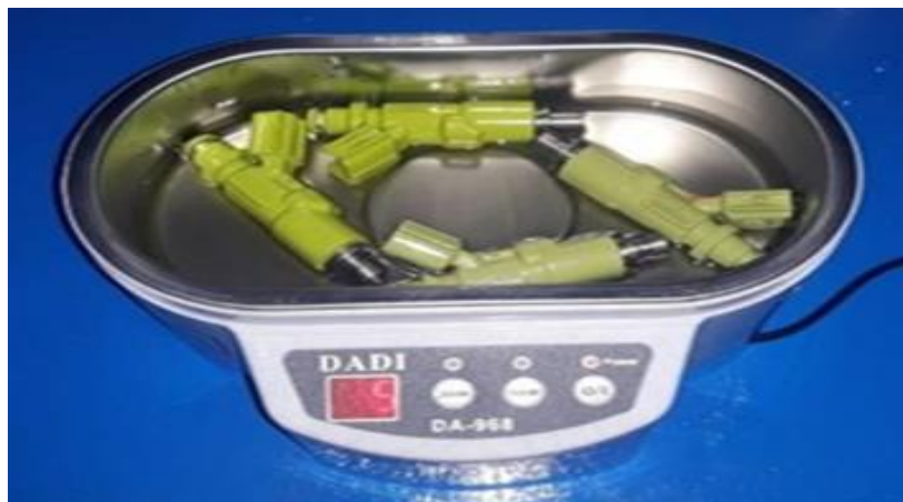
Figure 5. Results of Cleaning Injectors Using Ultrasonic Waves
